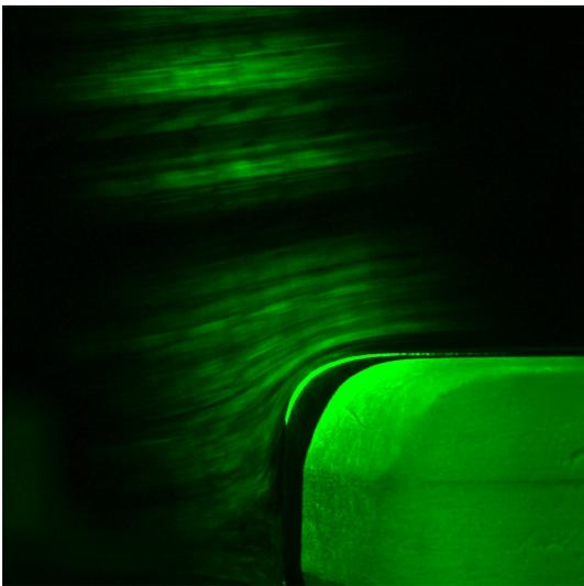
Figure 11: The simulated streamlines, Bello, on the flow visualization with yaw angle of  $0^\circ$  on the model face.
